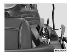
(1) Position Control Lever (A) Lifting
