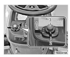
(1) Turn Signal Light Switch(2) Head Light Switch(3) Horn Switch
