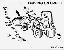
When driving uphill with a loaded bucket and rear ballast installed, keep the higher end of the tractor heavier. In other words, drive forward on uphill and backward on downhill.
