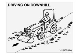
When driving on downhill with an empty bucket and rear ballast installed, keep the rear ballast toward the higher level of the ground. In other words, drive backward on uphill and forward on downhill.
