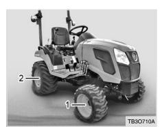
(1) Front Wheel Bolt / Nut (2) Rear Wheel Bolt / Nut
