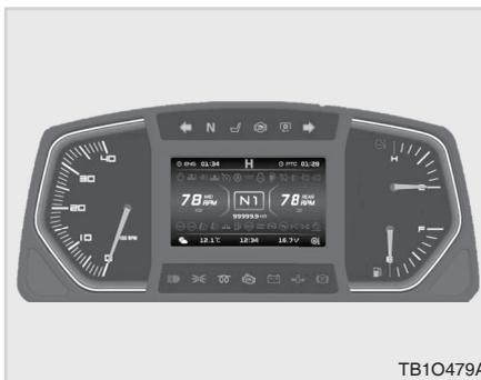
When first started, all needles on the instrument panel move to the highest point and then return to their original position. If the engine is restarted before a certain period of time after stopping, this function does not operate.
