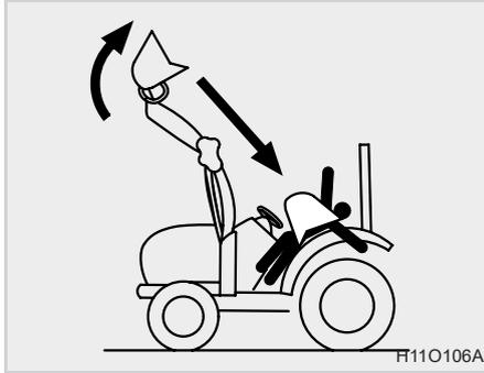
5. Before disconnecting the loader or attaching a loader to the tractor, visually inspect the unit and confirm there are no loose or missing hardware, leaks or other items that may require repair. Also carefully inspect the loader to make sure the locking handles and mechanism are in the “locked” position and the attachment (bucket, forks, etc.) is securely and properly connected to the loader.
