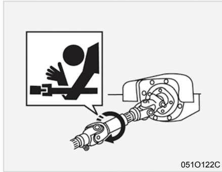
4. When operating stationary PTO driven equipment, always apply the tractor parking brake and place chocks behind and in front of the rear wheels. Stay clear of all rotating parts.
