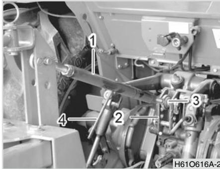
7. Install the top link to the top link hole of the implement. Loosen the lock nuts of top link and turn the top link handle to adjust the length of it as needed. Align the pin holes for top link and top link hole on the implement to insert the set pin. Insert the snap pin into the set pin hole securely to hold the set pin.
