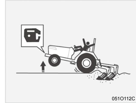
12. If the front of the tractor tends to rise up when heavy implements are attached to the three point hitch, weights should be installed on the tractor. Do not operate the tractor with a light front end.
