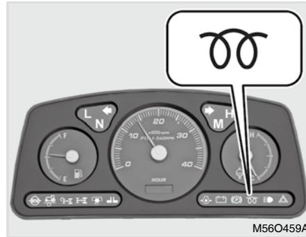
This indicates the operating condition of the preheat system. When the key switch is turned to the "ON" position, this indicator comes on for approx. 8 seconds. It is recommended to start the engine as soon as this indicator goes off for best starting performance. This indicator may not turn on if the engine is warm. In this case, the engine can be started without the preheat operation.
