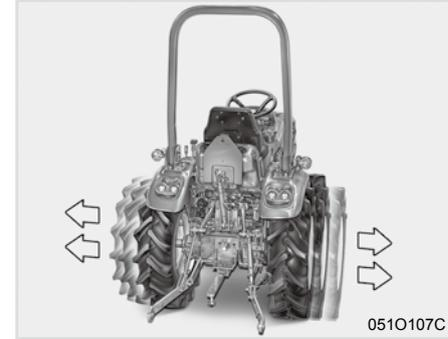
21. Extra caution should be taken when driving tractors with narrow tread widths. For added stability you should adjust your rear wheel tread width, see page 4-25.
