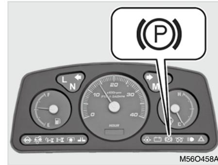
When the parking brake is actuated, the lamp lights "ON".
