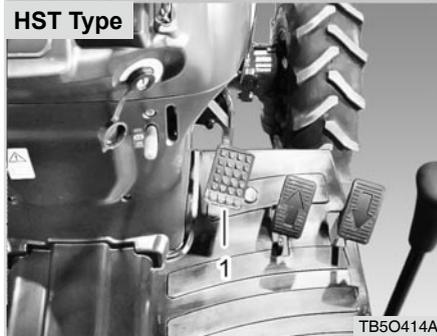
(1) Brake Pedal                      (2) Pedal Interlock
