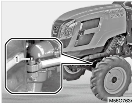
(1) Steering cylinder end nipple (LH/RH)
