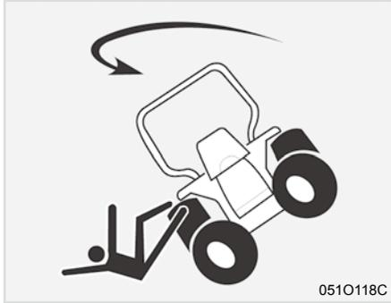
2. Always slow the tractor before turning. Turning at high speed may tip the tractor over or cause an operator to lose control of the tractor.
