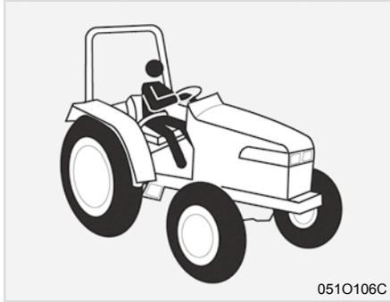
19. Before starting your tractor you should depress the clutch and make sure that all shift levers are in the neutral position and parking brake is applied.
