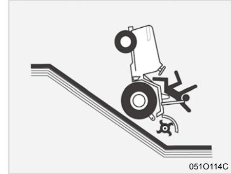
19. Driving forward out of a ditch or steep inclines can cause the tractor to tip over backwards. To avoid this you should back out of these positions. Four wheel drive tractors can give you a false sense of security in the tractors ability to maneuver out of these positions, so extra caution should be taken.
