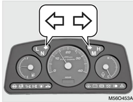
Operating the turn signal lamp switch turns on the corresponding lamp in green.
