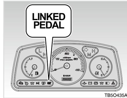
The lamp comes on when the synchronization switch or lever is connected.
