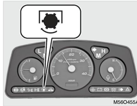
This indicator shows the PTO engagement condition. When the PTO is engaged, this indicator comes on. When the PTO clutch is disengaged, this indicator goes off.
