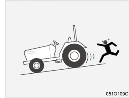
3. Do not park your tractor on a steep incline, and remember to shut off the engine and PTO before dismounting the tractor.
