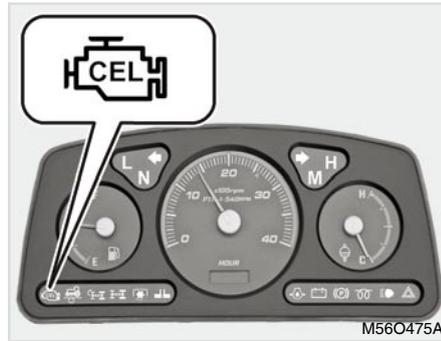
This warning lamp comes on when any major electric device or engine fuel system is malfunctioning. When this warning lamp is illuminated, make sure to stop the engine immediately and have the engine checked.
