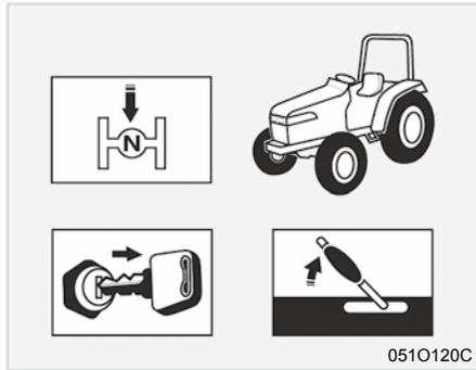
1. Disengage the PTO, lower all implements, place all control levers in the neutral position, set the parking brake, stop the engine and remove the key.
