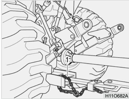
9. Check for correct coupling between tow hook and trailer. See the Towing Attachments chapter.
