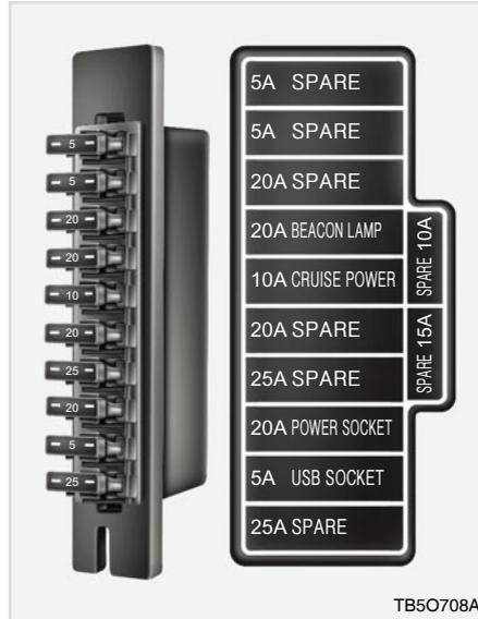
3. If the fuse is blown, replace it with a new fuse with same capacity. Make sure it is firmly installed.
