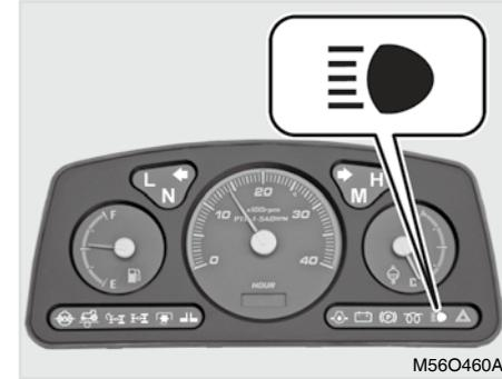
This lamp comes on in blue when the high beam head light is switched on. Driving with high beam head light disturbs an approaching vehicle's visibility. For safe driving, use the high beam head light only if necessary.
