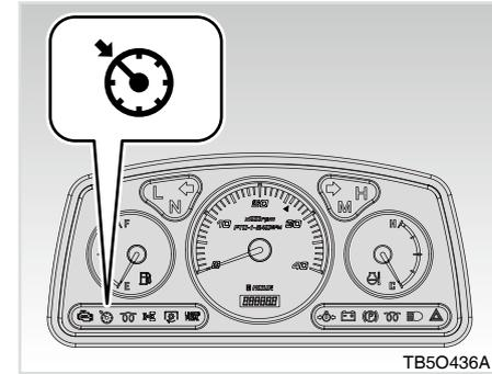
To activate the cruise control function, set the desired speed and press the switch to the "ON" position.
