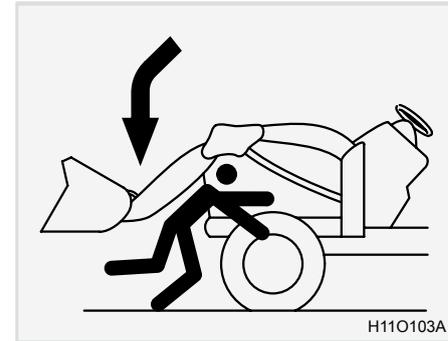
2. Do not stand under the lifted loader or get close to it. Also, lower the loader arm onto the ground before leaving the tractor. Otherwise, it may lead to a fatal injury or even death.
