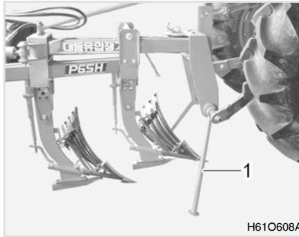
8. Raise up the implement by position control of tractor. Remove the implement support as needed. Align the implement by adjusting the length of the check chains on both sides. Tighten the lock nuts on the check chain securely.
