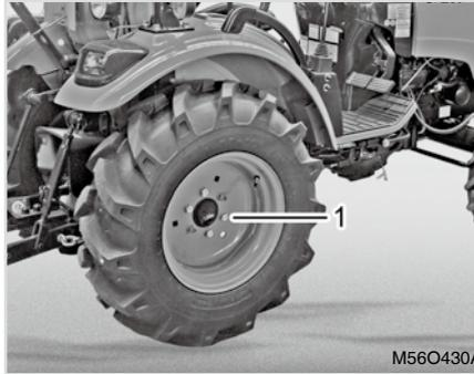
(1) Tightening torque: 20.0 ~ 23.0 kgf·m
