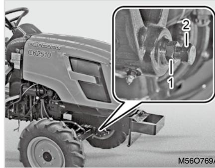
*(1) Lock Nut      (2) Adjusting Bolt*
