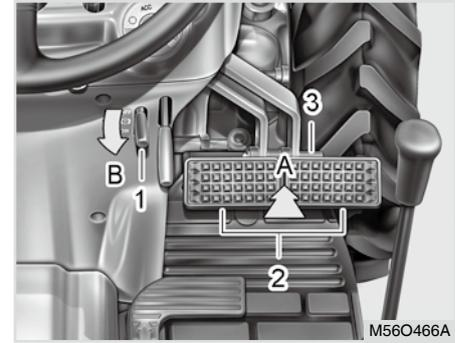
(1) Foot Parking Brake Lever                      (3) Pedal Interlock
