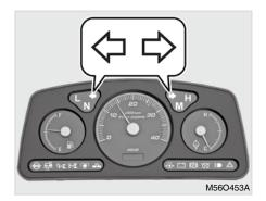
Operating the turn signal lamp switch turns on the corresponding lamp in green.
