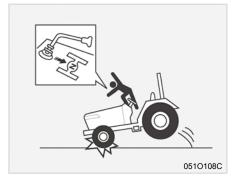
2. Avoid accidental contact with gear shift levers while the engine is running. Unexpected tractor movements can result in bodily injury.
