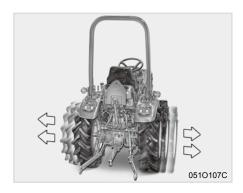
21. Extra caution should be taken when driving tractors with narrow tread widths. For added stability you should adjust your rear wheel tread width, see page 4-25.
