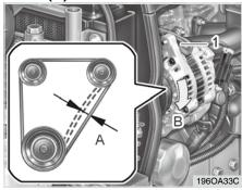
(1) Adjusting Bolt (A) Adjusting Belt Tension
