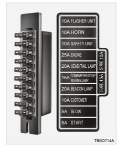
There are marks for the fuse capacity and location on the cover of the fuse panel. Replace the fuse according to the following procedure:
