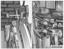
(1) Double Acting Valve 1 & Lever 1 (A) Port A (B) Port B
