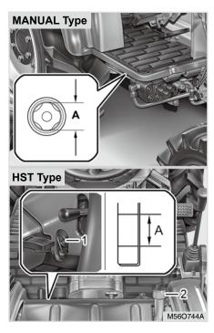
(1) Gauge (2) Oil Filler Plug (A) Oil level is acceptable within range
