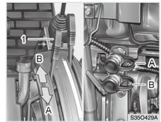
(1) Double Acting Valve Lever (A) Port A (B) Port B
