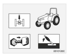
Disengage the PTO, lower all implements, place all control levers in the neutral position, set the parking brake, stop the engine and remove the key.
