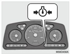
This lamp comes on when the engine oil pressure or oil level is low.
