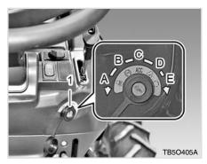
(1) Key switch (C) ACC (A) Pre-heat (D) ON (B) OFF (E) Start
