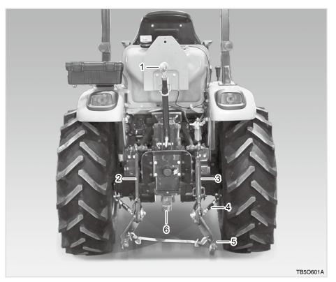
(1) Top Link (2) Lift Rod (L) (3) Lift Rod (R) (4) Check Link
