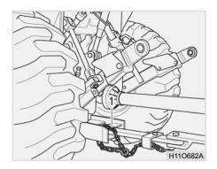
ing the proper adaptor parts, attach the chain to the tractor draw-bar support or other specified anchor location. Provide only enough slack in the chain to permit turning. See your Dealer for a chain with a strength rating equal to, or greater than the gross weight of the towed machine.
