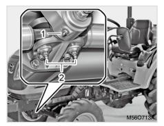
(1) Front Bracket (2) Steering Cylinder Support Pin Nipple (LH/RH)
