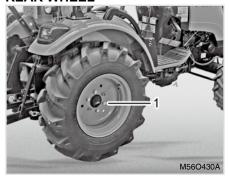
(1) Tightening torque: 20.0 ~ 23.0 kgf·m
