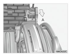
(1) Position Control Lever (A) Lifting
