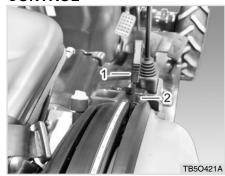
(1) Hydraulic Control Lever (2) Lock Bolt
