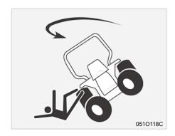
Always slow the tractor before turning. Turning at high speed may tip the tractor over or cause an operator to lose control of the tractor.
