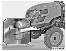
(1) Steering cylinder end nipple (LH/RH)
