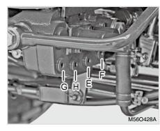
G: Boom Up H: Boom Down E: Bucket Up (Roll back) F: Bucket Down (Dump)
