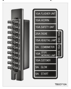
2. Open the fuse box cover and check the fuse in question using fuse tongs.
