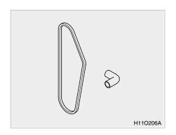
Belts, hoses and boots, which are made of rubber, get weakened and cracked as they age. If these parts remain in this state, they can be broken off, leading to a serious problem in the tractor. Therefore, regularly check or replace those items to prevent the failure.
