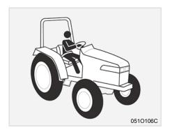
19. Before starting your tractor you should depress the clutch and make sure that all shift levers are in the neutral position and parking brake is applied. 20. For your safety **ROPS** with a seat belt is recommended for all applications.
