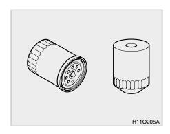
Filters for the engine, transmission, air cleaner, and A/C are consumables that purify oil and air. Make sure to replace the these items when changing oil.
