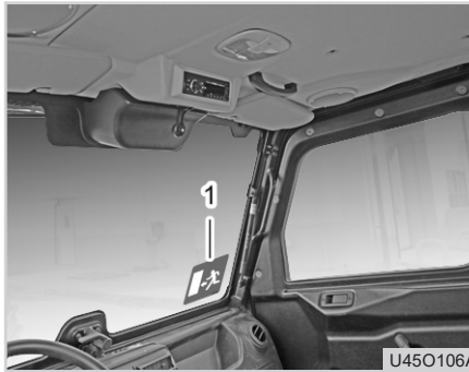
(1) Emergency Exit Label
