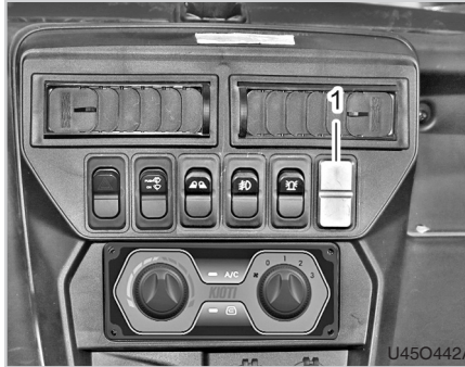
(1) Spare Switch Panel
