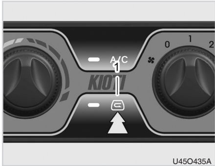
(1) Ventilation port changeover switch
