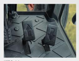
**HST Pedals**Allows for seamless on-the-go direction changes, keeping
