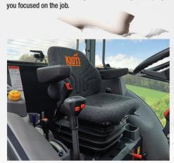
**Deluxe suspension seat**Provides a comfortable ride for the operator, even on rough terrain.
