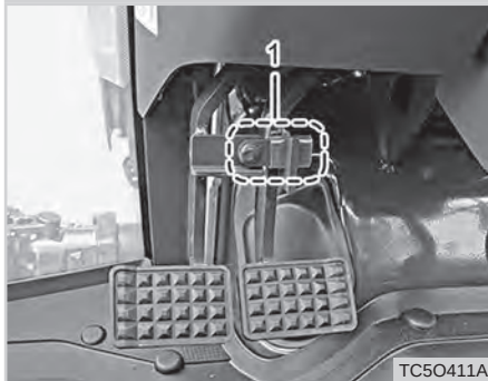
(1) Pedal Interlock Latch
