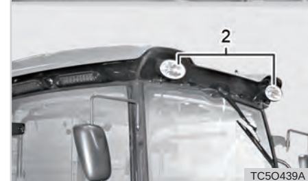
(1) Working Light Switch (2) Working Light
