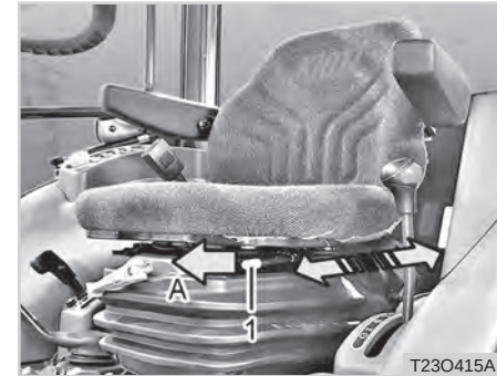
(1) Seat Adjustment Lever (A) Pull
