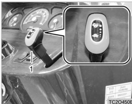
(1) Hand Throttle Lever 🐢 : Slow 🐘 : Fast
