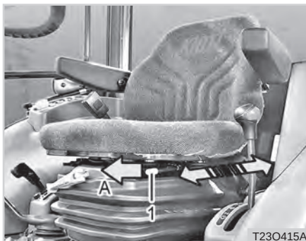
(1) Seat Adjustment Lever (A) Pull
