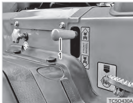
(1) Front Wheel Drive Lever (4WD)
