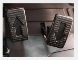
Twin HST Pedals Twin HST pedals enable easy forward and reverse movement, with smooth acceleration and deceleration. The dual pedals simplify operation, reducing operator fatigue during long hours of work and repetitive tasks.
