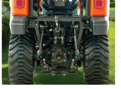
Mid and Rear PTO Operate the rear and mid PTO's independently or simultaneously reducing downtime to change implements ensuring uninterrupted productivity.
