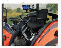
Factory Installed Cab Enjoy unmatched comfort with a factory-installed, climatecontrolled cab featuring heat and ac, premium suspension seat, wide operator station, increased storage and reduced noise and vibration.
