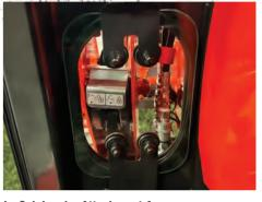
**In-Cab Loader Attachment Access** Enjoy the convenience and safety of managing the loader quick release from the comfort of the cab, eliminating the need to repeatedly get on and off the tractor.
