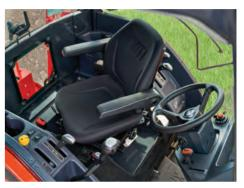
Swivel Seat for Backhoe Operation (Optional) The swivel feature allows the operator to rotate the seat towards the rear of the tractor, facilitating in-cab operation of the backhoe when installed.
