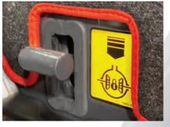
**Rear Differential Lock** The lever easily engages the differential, ensuring optimal traction in slippery conditions like uneven or muddy terrain.
