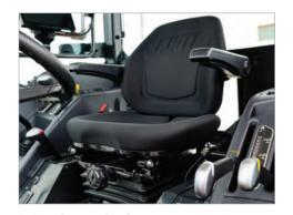
Deluxe Suspension Seat The Deluxe Suspension Seat is engineered to deliver comfort for the operator by absorbing shocks and vibrations, minimizing the impact of rough surfaces and ensuring a smooth ride.
