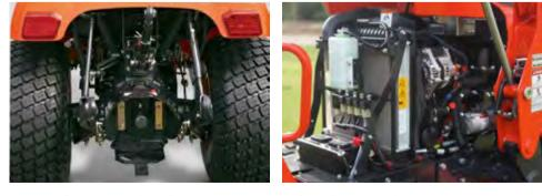
**Rear PTO and 3-Point Hitch** installation.
