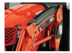
Self-Leveling Loader (Optional) Maintains the desired bucket angle when lifting and lowering, preventing the need to manually position the bucket throughout the lift/lower cycle to keep your material in the bucket. This can increase productivity while adding a layer of safety to your worksite.
