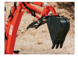
Electric / Hydraulic Thumb (Optional) Designed for ease of use, this feature allows for precise and responsive control of the hydraulic thumb directly through the joystick, allowing you to accomplish more in less time.
