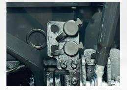
Rear Hydraulic Remotes A standard single remote valve, with an optional second valve, accommodates a wide range of attachments and implements (SE models only)
