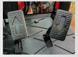
HST Pedals Allows for seamless on-the-go direction changes, keeping you focused on the job.
