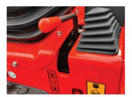
Four-Wheel Drive Four-wheel drive comes standard on all models and is engaged with a simple push-pull lever.
