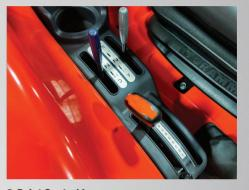
3-Point Control Lever Provides convenient raising and lowering of the lift arms, simplifying implement attachment. (SE models only)
