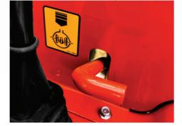
**Rear Differential Lock** The lever easily engages the differential, ensuring optimal traction in slippery conditions like uneven or muddy terrain..
