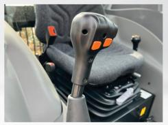
Single Lever Joystick The lever returns to neutral when released. A float position enables the bucket to float freely over the ground surface. (SE models only)
