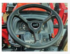
**Power and Tilt Steering** Standard power steering reduces effort for tight, repetitive turns. The tilting steering wheel adjusts easily with a push of a lever to fit operator needs.
