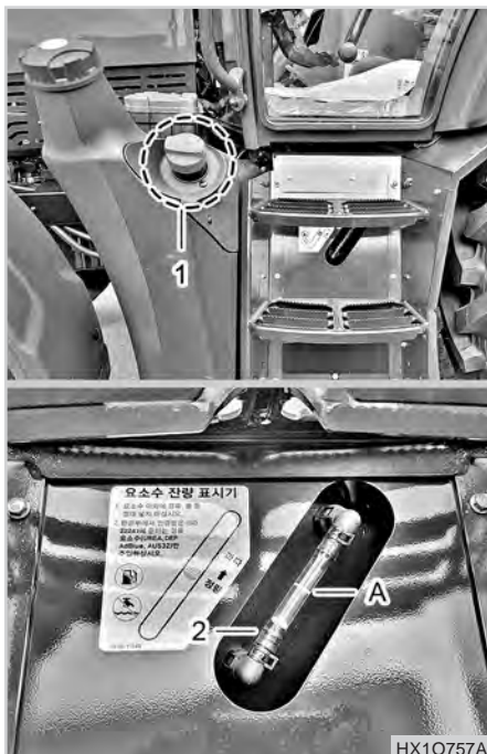
(1) DEF fill cap (2) DEF level gauge (A) Proper DEF level
