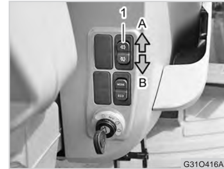
(1) DPF Regeneration Switch (A) Activation (B) Deactivation
