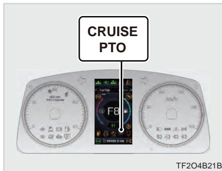
The cruise PTO can set the engine RPM's and enable to operator to increase/decrease by 50 RPM's each time the +/- switch is depressed.
