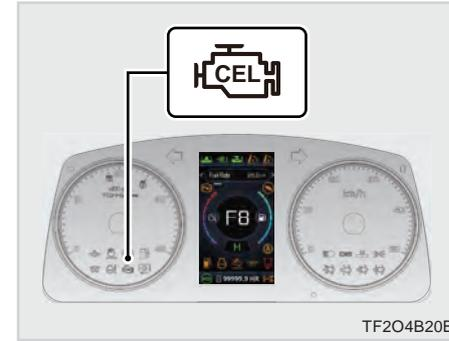
The CEL lamp illuminates on the dash board when the ECU recognizes any malfunction or loss of signal from any engine or fuel sensor.
