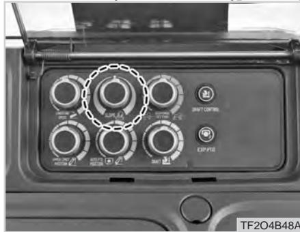
This dial is used to adjust the height of the lift cylinder on inclination.
