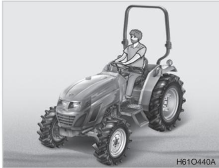
This tractor is designed for use in agricultural settings and applications. This tractor should be used in conjunction with equipment designed and manufactured for agricultural applications that are intended to be pulled by a drawbar or attached to a 3-point hitch of the proper size and category matching to this unit and if needed, powered by a type one 540 RPM shaft or a type two 1,000 RPM shaft.
