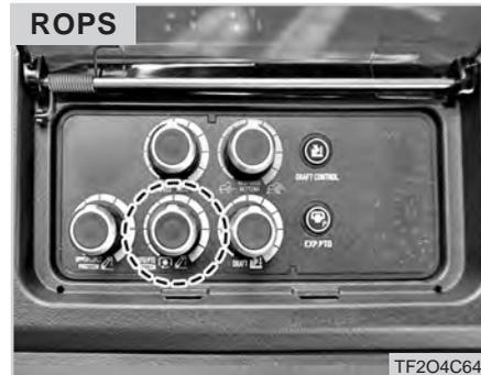
Adjusts the upper limit for the lower links to turn the PTO off "automatically" when the three-point is raised while operating the PTO in the "auto" mode. When the three-point is lowered, the same set-point will "automatically" turn the PTO back on.
