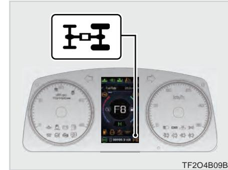
When the 4wd is engaged, the 4WD lamp illuminates on the dashboard. The 4WD can be engaged with the 4WD switch.
