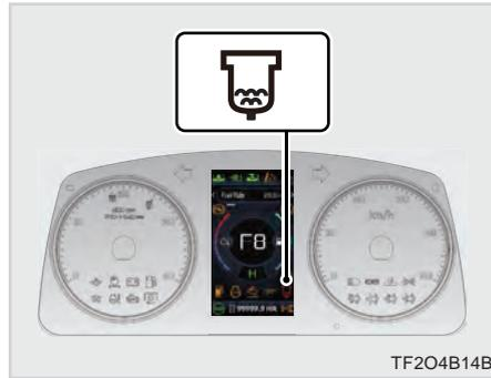
When approximately 5 ounces of water (45 cc) is accumulated in the fuel filter, the water in fuel warning lamp will illuminate on the dashboard.
