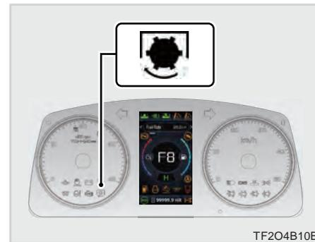
When the PTO is engaged, the PTO lamp illuminates on the dashboard. When starting the tractor, the PTO must be in the off position. When standing up from the seat with the PTO on, the parking lamp will illuminate, and the ignition will be turned off 2 seconds after the buzzer sounds.
