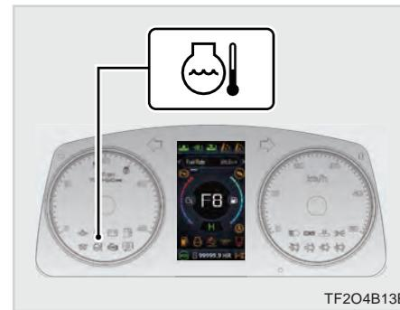
If the coolant temperature is 239°F or above 239°F (115°C) for more than 5 seconds, buzzer is heard and lamp is turned on. Stop the engine, contact a **KIOTI** dealer immediately.
