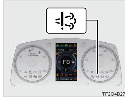
The emission warning lamp will illuminate on the dashboard when an error or malfunction with the emissions system is detected.
