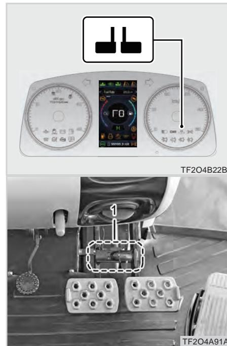
(1) Brake Pedal Lock (Both Sides)
