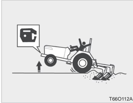
11. If the front of the tractor tends to rise up when heavy implements are attached to the three point hitch, weights should be installed on the tractor. Do not operate the tractor with a light front end.
