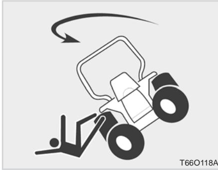
2. Always slow the tractor before turning. Turning at high speed may cause a loss of control or tractor roll-over.
