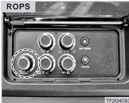
It sets the upper limit for the lower links when using the lift/lower switch, the Turn/lift function or the Reverse/lift function.
