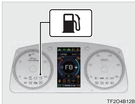
The fuel level warning lamp will illuminate on the dashboard when the fuel level in the tank drops below a safe operating level.
