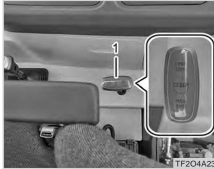
(1) Creep gear speed lever
