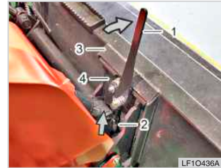
(1) Hand lever (2) Locking pin (3) Bucket slot (4) Attachment holder
