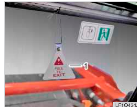
(1) Emergency exit tag
