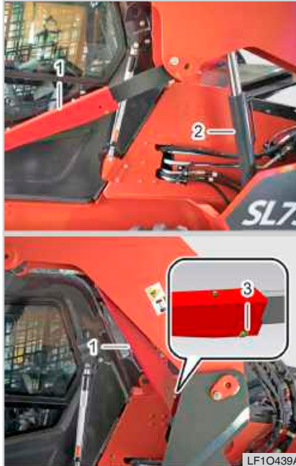
(1) Boom lock (3) Snap pin
