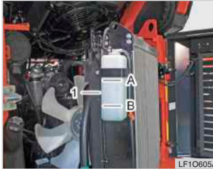
(1) Reservoir Tank (A) FULL (B) LOW
