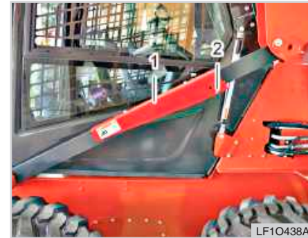
(1) Boom lock (2) Locking pin
