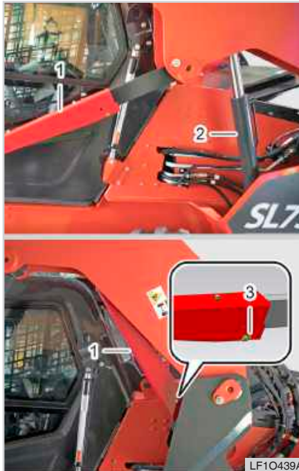
(1) Boom lock (3) Snap pin
