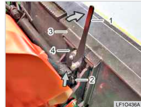
(1) Hand lever (2) Locking pin (3) Bucket slot (4) Implement holder
