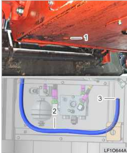
(1) Drain hole (2) Drain hose (3) Plug
