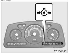
This lamp comes on when the engine oil pressure or oil level is low.
