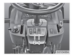
(1) PTO Cruise Switch (2) PTO Cruise Control Switch
