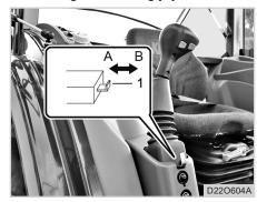
(1) Joystick Lock Lever (A) Lock (B) Unlock
