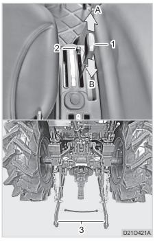
(1) Position Control Lever (2) Lock Bolt
