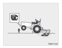
12. If the front of the tractor tends to rise up when heavy implements are attached to the three point hitch, weights should be installed on the front of tractor. Do not operate the tractor with a light front end.
