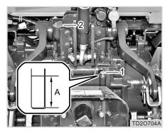
(1) Oil Dipstick (2) Oil Filler Plug (A) Oil Level Is Acceptable Within This Range
