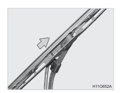
Lift the wiper blade to its end and install it so that the fixing lever is engaged with the wiper arm. (A clicking sound is heard)
