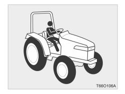
19. Before starting your tractor you should depress the clutch and make sure that all shift levers are in the neutral position and parking brake is applied. 20. For your safety **ROPS** with a seat belt is recommended for all applications.
