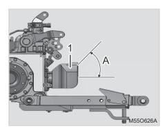
(1) PTO Cover (A) Allowable Angle Of Universal Joint: 50°
