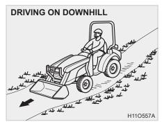
When driving downhill with the empty bucket and rear ballast installed, keep the rear ballast toward the higher level of the ground. In other words, drive backward on uphill and forward on downhill.
