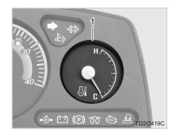
(1) Coolant Temperature Gauge C: Cold H: Hot
