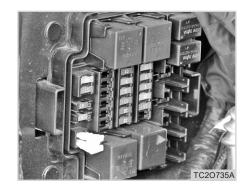
The fuse panel is located in the right section of the engine compartment.
