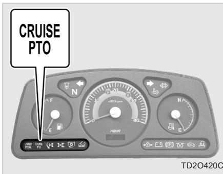
The switch is used to set the PTO rpm. With the PTO cruise button set in the ON position, pressing the SET (-) button turns on this lamp.
