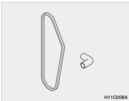
Belts, hoses and boots, which are made of rubber, get weakened and cracked as they age. If these parts are kept left in this state, they can be broken off, leading to a serious problem in the tractor. Therefore, regularly check or replace those items to prevent the failure.
