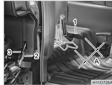
(1) Brake Pedal (2) Clutch Cable
