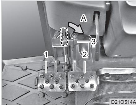
(1) Brake Pedal (Lh)    (2) Brake Pedal (Rh)
