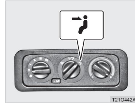
Air flows out from four left and right vents toward the driver when turning the vent mode dial to the (
