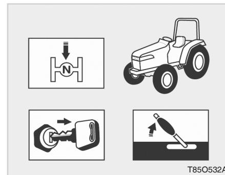
1. Make sure to reduce the engine rpm before stopping the engine.
