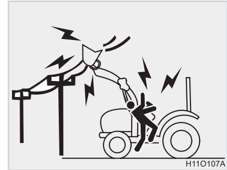
6. Do not allow loader arms or attachment to contact electrical power lines. Electrocutation will cause serious injury or death.
