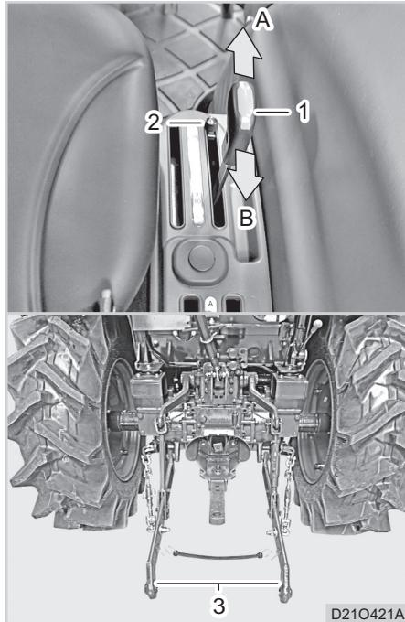
(1) Position Control Lever (2) Lock Bolt
