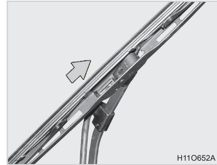
3. Lower the blade and pull out the blade by moving it in the shape of "U". (Arrow direction in the figure)
