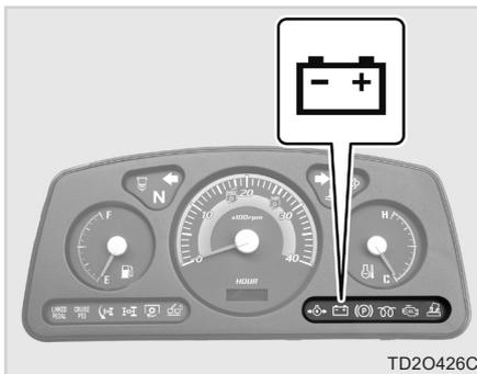
This lamp is turned On when the starting switch is turned On before starting the engine but turned Off after starting the engine.
