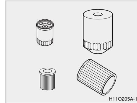
Filters for the engine, transmission, air cleaner, and A/C are consumables that purify oil and air. Make sure to replace these items when changing oil.
