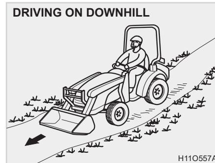
When driving downhill with the empty bucket and rear ballast installed, keep the rear ballast toward the higher level of the ground. In other words, drive backward on uphill and forward on downhill.
