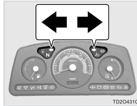
Operating the turn signal lamp switch left and right turns on the corresponding lamp in green.
