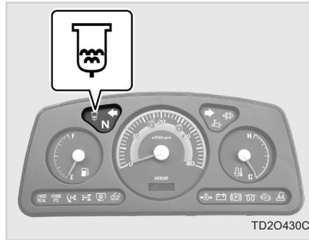
When a certain amount of water (Approx. 45 cc) is accumulated in the fuel filter, this lamp will be turn on. In this case, stop the engine immediately and drain water from the fuel filter.
