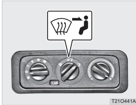
Air flows out from four front and four left and right vents when turning the vent mode dial to the Bi-level (
