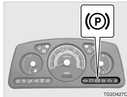
When the parking brake is actuated, the lamp lights On.
