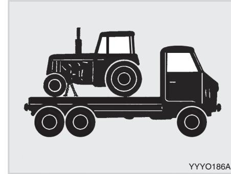
4. It is recommended to back the tractor onto the transporting vehicle and drive the tractor OFF in the forward direction.
