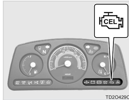
This lamp indicates the current condition of the engine. If this comes on while the engine is running or during working, contact your dealer.
