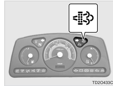
If carbon is accumulated in the exhaust catalytic filter, this warning lamp comes on or blinks.
