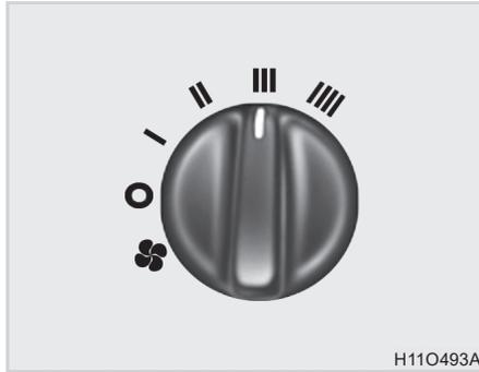
The fan speed for the heater and air conditioner can be adjusted in four positions.
