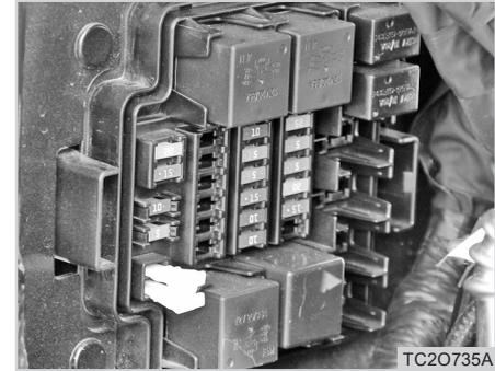
The fuse panel is located in the right section of the engine compartment.
