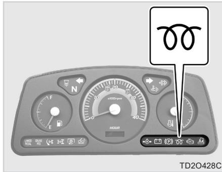
This indicates the operating condition of the preheat system. In case the auto pre-heating kit is installed, this indicator comes on 8 seconds when the key switch is turned to the “ON” position. In case of basic model, this indicator comes on when the key is held in “PRE-HEAT ” position by operator.
