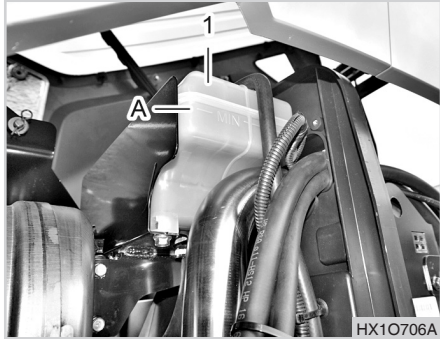
(1) Reservoir Tank (A) Min (Lack)
