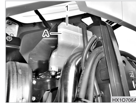
(1) Reservoir Tank (A) MIN (Lack)
