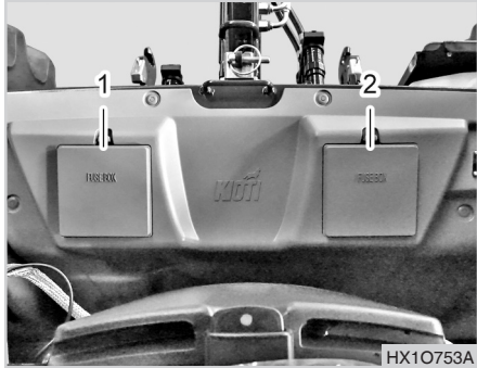
(1) Fuse Box 1 (2) Fuse Box 2
