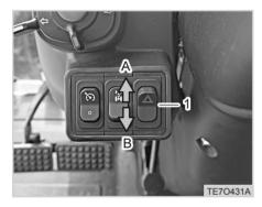
(1) Hazard Lamp Switch (A) ON (B) OFF
