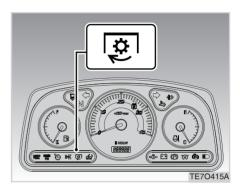
This indicates the operating condition of the preheat system. When the key switch is turned to the "ON" position, this lamp comes on. It is recommended to start the engine as soon as this lamp goes off for best starting performance. This lamp may not turn on if the engine is warm. In this case, the engine can be started without the preheat operation.
