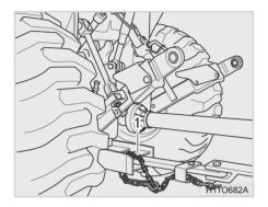
Using the proper adaptor parts, attach the chain to the tractor draw-bar support or other specified anchor location. Provide only enough slack in the chain to permit turning. See your Dealer for a chain with a strength rating equal to, or greater than the gross weight of the towed machine.
