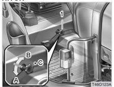
(1) 3-point hitch lowering speed knob (A) "FAST" (C) "LOCK"
