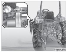
(1) Grease Fitting (Power steering cylinder) (RH, LH)
