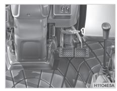
(1) Brake Pedal Lock (Both Sides)
