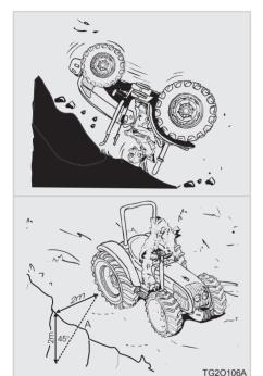
When operating near ditches and banks, always keep your tractor behind the shear line. Avoid ditches, embankments and river-banks which might cave in.
