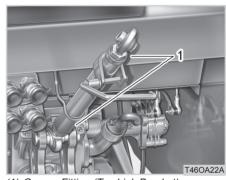
(1) Grease Fitting (Top Link Bracket)
