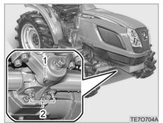
(1) Grease Fitting (Front bracket axle pivot)
