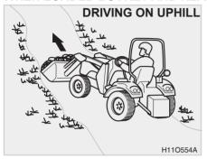
When driving on uphill with the loaded bucket and rear ballast installed, keep the higher end of the tractor heavier. In other words, drive forward on uphill and backward on downhill.
