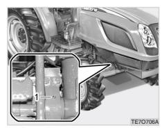
(1) Grease Fitting (Rear Bracket Axle Pivot)
