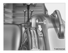
(1) Position Control Lever (A) Lifting
