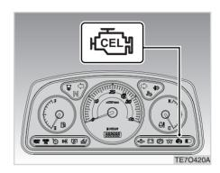
If carbon is accumulated in the exhaust catalytic filter, the warning lamp comes on or blinks.
