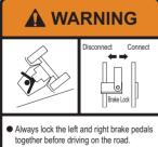
Activating only one brake at higher speeds could cause loss of control.
