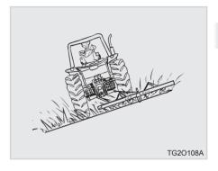
• If you need cross a steep slope, do not steer uphill, but slow down and take a wide turn. Always drive straight up or down a slope, never across it. When travelling up or down a slope, keep the heavy end of the tractor and the implement pointed uphill.
