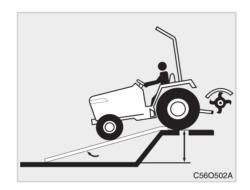
5. It is recommended to use the 4WD and drive backward when moving onto a bank.
