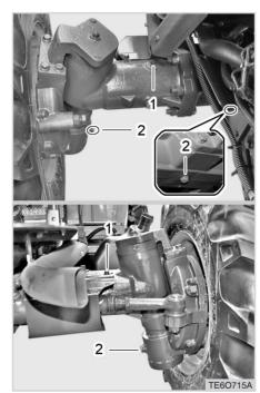
(1) Check & Filling Plug (2) Drain Plug
