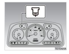
The warning buzzer sounds when (approx. 45 cc) of water is accumulated in the fuel filter. In this case, stop the engine immediately and drain water from the fuel filter.
