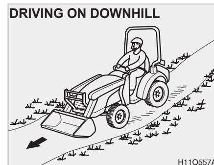
When driving on downhill with the empty bucket and rear ballast installed, keep the rear ballast toward the higher level of the ground. In other words, drive backward on uphill and forward on downhill.
