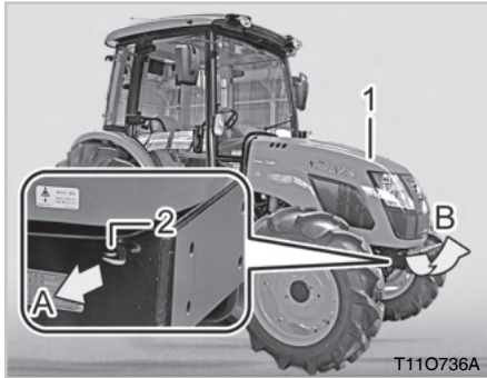
(1) Hood (A) Pull (2) Opening Knob (B) Lift
