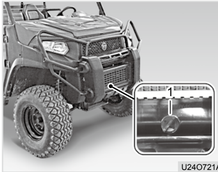
(1) Coolant drain plug of radiator
