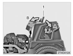
(1) Parking Brake Lever(A) Engaged(B) Disengaged
