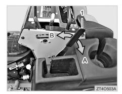
(1) Parking Brake Lever(A) Engage(B) Disengage
