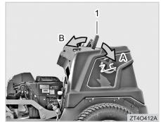
(1) Parking Brake Lever (A) Engaged (B) Disengaged
