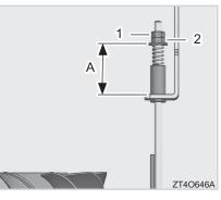
(1) Lock Nut (2) Adjusting Nut (A) 56mm ±5 (Length Adjustment)
