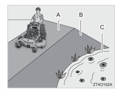
(A) Safe Range (Slope less than 15 degrees)
