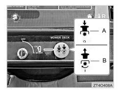
(1) PTO Switch (A) Disengage
