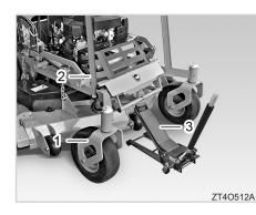
(1) Cast Support Assembly(2) Rope(3) Jack
