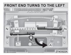
(1) LH Steering Levers(2) RH Steering Levers(A) Reverse Right Turn
