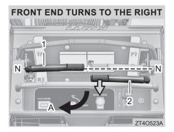
(1) LH Steering Levers(2) RH Steering Levers(A) Reverse Left Turn
