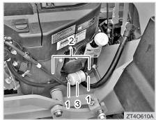
(1) Pipe Clamp(2) Fuel Line(3) Fuel Filter
