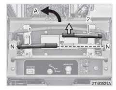
(1) LH Steering Levers(2) RH Steering Levers(A) Forward Left Turn
