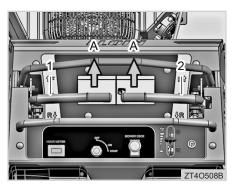
(1) LH Steering Levers (2) RH Steering Levers (A) Forward
