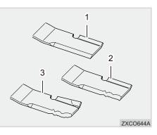
(1) New Blade(2) Worn Blade(3) Cracked Blade
