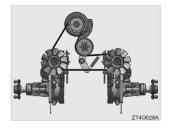
3. Make sure the axle belt path is correct and the belt is aligned in all pulleys correctly.
