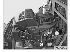
(1) Air Intake Screen (2) Engine Shroud
