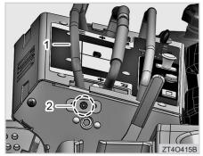
(1) Reference Control Front Lever (2) Adjust Bolt
