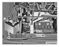
(1) Dead Battery (2) Jumper Cables (-) (3) Jumper Cables (+) (4) Helper Battery
