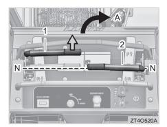
(1) LH Steering Levers(2) RH Steering Levers(A) Forward Right Turn
