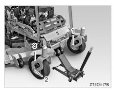
(1) Nut(2) Wheel Bolt(3) Wheel Support Fork Bracket
