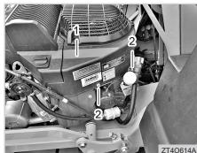
(1) Engine Shroud (2) Mounting Bolt
