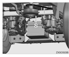
(1) PTO Belt (2) Engine Pulley
