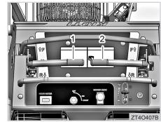
(1) LH Steering Lever (2) RH Steering Lever
